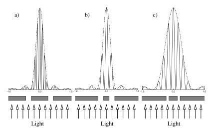
Fig. 5.3. Fraunhofer diffraction pattern of three different double apertures, from left to right, first the separation between the apertures has been decreased, then - on the right hand side - the diameter of the apertures has been decreased.
