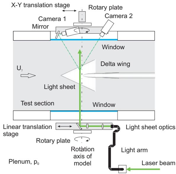
**Fig. 9.44.** Stereoscopic PIV arrangement inside the perforated test section of the transonic wind tunnel DNW-TWG showing the coated delta-wing and light sheet.
