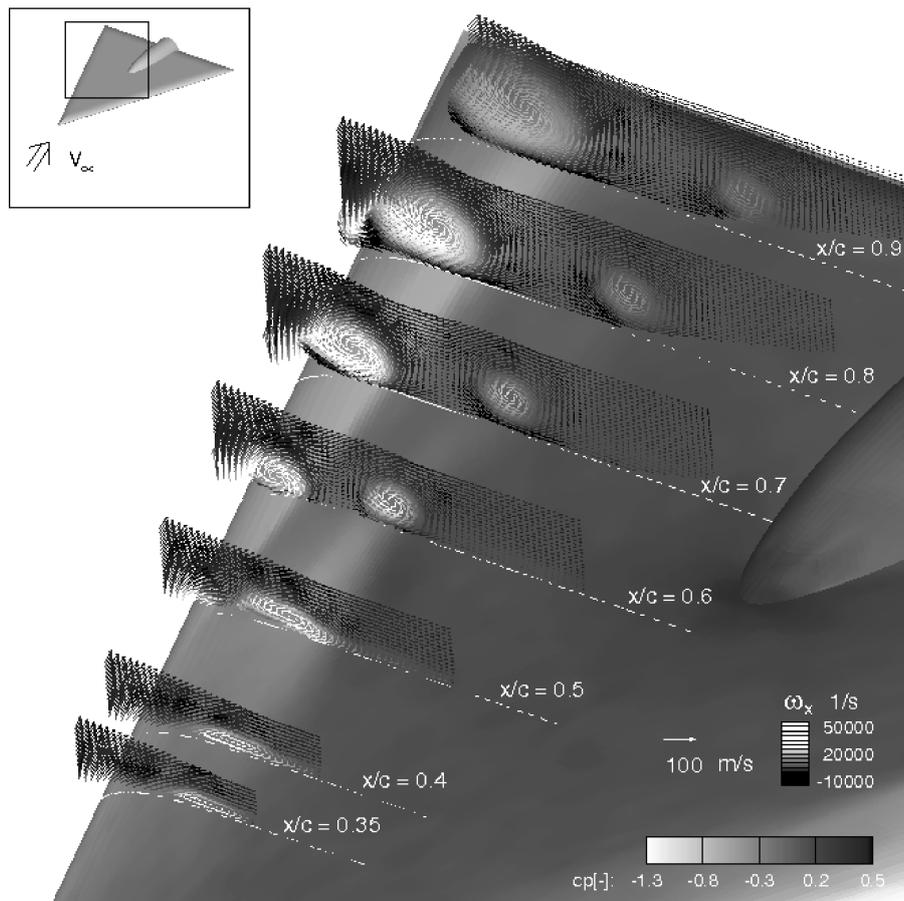
**Fig. 9.45.** Time averaged pressure, velocity and vorticity distributions above the delta wing with rounded leading edges for  $\alpha = 13.3^\circ$ ,  $Ma = 0.4$  and  $R_{MAC} = 3 \cdot 10^6$ . The in-plane velocity vectors are plotted in different planes perpendicular to the delta wing axis. The gray levels of the vectors correspond to the out-of-plane vorticity. The gray levels at the surface are related to the local pressure coefficient.
