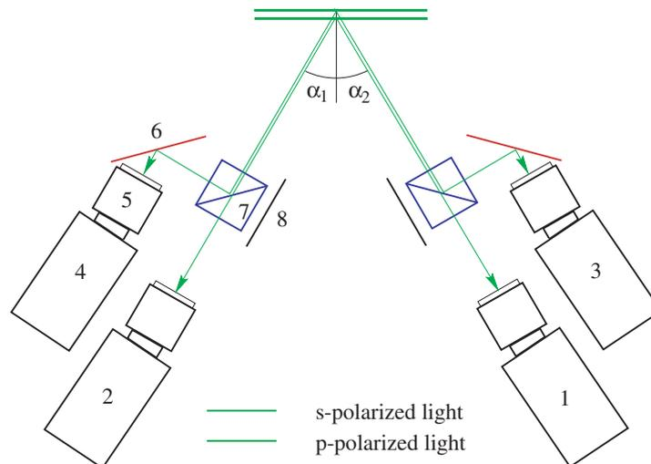
**Fig. 9.85.** Schematic setup of the recording system. 1-4 digital cameras, 5 lens, 6 mirror, 7 polarizing beam-splitter cube with dielectric coating between the two right-angle prisms, 8 absorbing material,  $\alpha$  opening angle.
