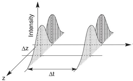
**Fig. 9.88.** Timing diagram for the simultaneous determination of all three velocity components in spatially separated planes.
