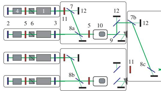
**Fig. 9.86.** Four-pulse four frequency Doppler laser system. 1 Pump cavity, 2 Full reflective mirror, 3 Partially transmitting mirror, 4 Pockels cell, 5  $\lambda/4$  retardation plate, 6 Glan-Laser polarizer, 7 Mirror, 8 Dielectric polarizer, 9 Dichroic mirror, 10 Frequency doubler crystal with phase angle adjustment, 11  $\lambda/2$  retardation plate, 12 Beam dump.
