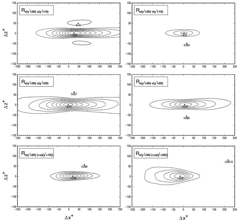
**Fig. 9.89.** Two-dimensional spatial cross-correlation function of fluctuating stream-wise ( $u$ ) with wall-normal ( $v$ ) velocity components measured at  $Re_\theta = 7800$ . *Top:*  $R_{v(y^+=20)u(y^+=10)}$  (left) and  $R_{u(y^+=20)v(y^+=10)}$  (right). *Centre:*  $R_{v(y^+=30)u(y^+=20)}$  (left) and  $R_{u(y^+=30)v(y^+=20)}$  (right). *Bottom:*  $R_{v(y^+=20)u(y^+=10)}$  with  $u > 0$  (left) and  $R_{v(y^+=30)u(y^+=20)}$  with  $u > 0$  (right).
