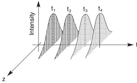
**Fig. 9.87.** Timing diagram for the temporally separated determination of all three velocity components. Different shading of the light-sheet profile indicates different states of polarization.
