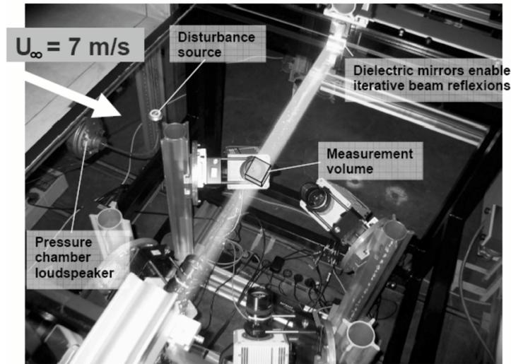
**Fig. 9.81.** Experimental setup at a flat plate boundary layer flow at a free stream velocity of  $U = 7$  m/s consisting of four Photron APX-RS CMOS cameras enabling time resolved tomographic PIV measurements of turbulent spots at the open test section of the 1m-wind tunnel of DLR Gttingen.
