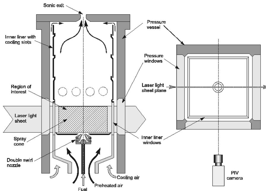
**Fig. 9.75.** Single sector pressurized combustion facility. Right: cross-sectional axial view.
