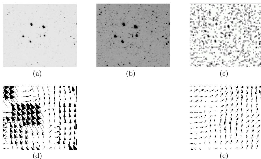
**Fig. 9.77.** Portion ( $120 \times 100$  pixel) of PIV recordings - inverted for clarity - and processed PIV data: a) fuel droplets, b) brightened version of a) with seeding visible, c) pre-processed image, d) flow field after standard PIV analysis, e) flow field obtained after enhancement of PIV images (from [377]).
