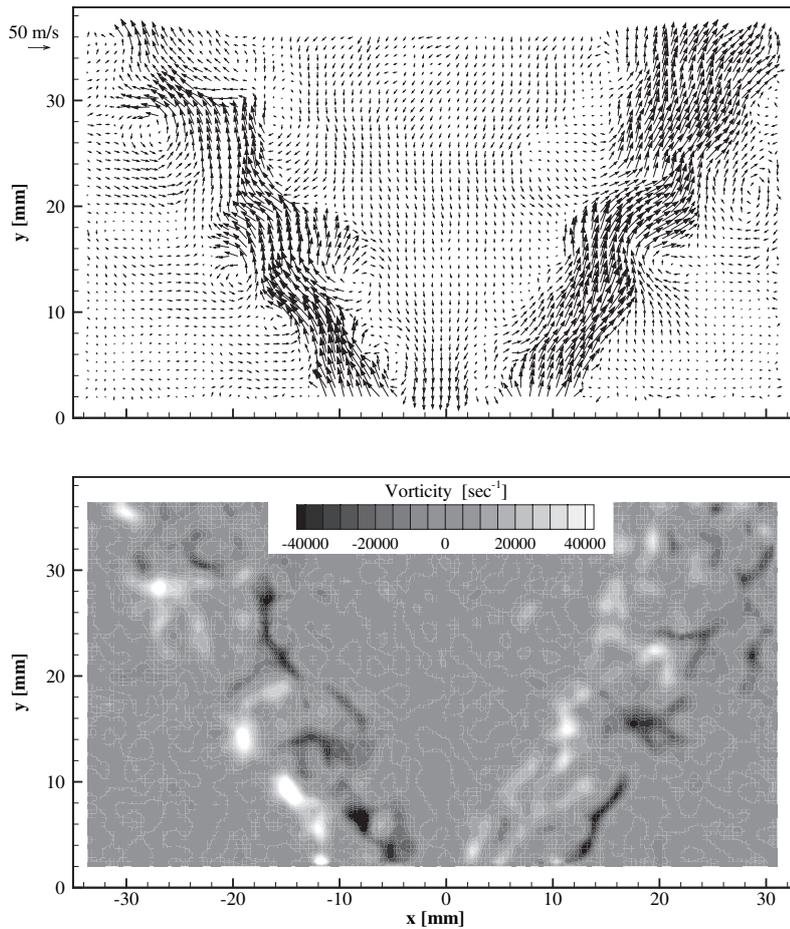
**Fig. 9.76.** Velocity map (top) and vorticity map (bottom) obtained at 3 bar.
