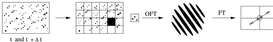
**Fig. 5.8.** Analysis of single frame/double exposure recordings: the hybrid (optical/digital) method utilizing the Young’s fringes technique.
