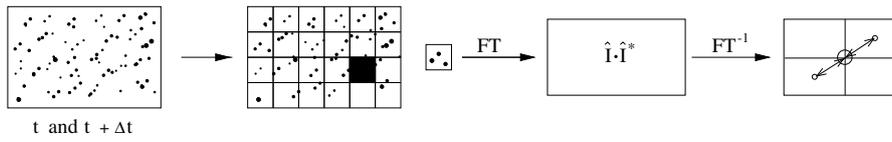
**Fig. 5.6.** Single frame/double exposure cross-correlation method flow chart.
