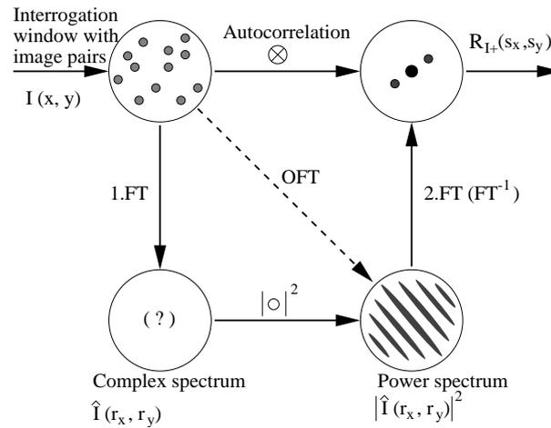
**Fig. 5.1.** Sketch of relation between 2D correlation function and spatial spectrum by means of the Wiener-Khinchin theorem. FT – Fourier transform,  $FT^{-1}$  – inverse Fourier transform, OFT – optical Fourier transform.
