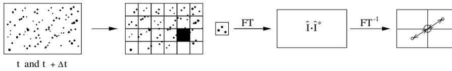
**Fig. 5.4.** Analysis of single frame/double exposure recordings: the fully digital autocorrelation method.
