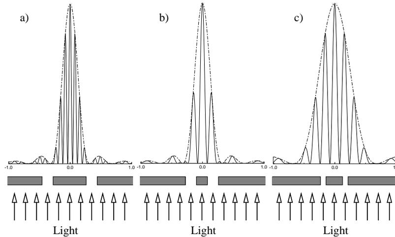
**Fig. 5.3.** Fraunhofer diffraction pattern of three different double apertures, from left to right, first the separation between the apertures has been decreased, then – on the right hand side – the diameter of the apertures has been decreased.
